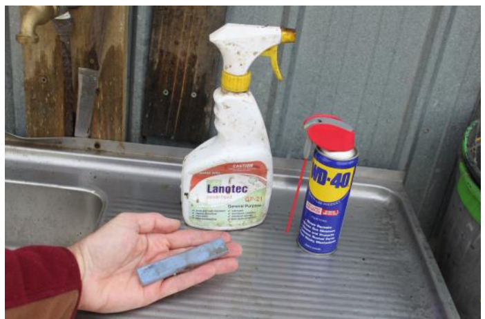
Felco grinding stone for sharpening knives and secateurs, Lanotec lanolin oil for oiling wooden handles and WD-40 for lubricating moving metal parts.
