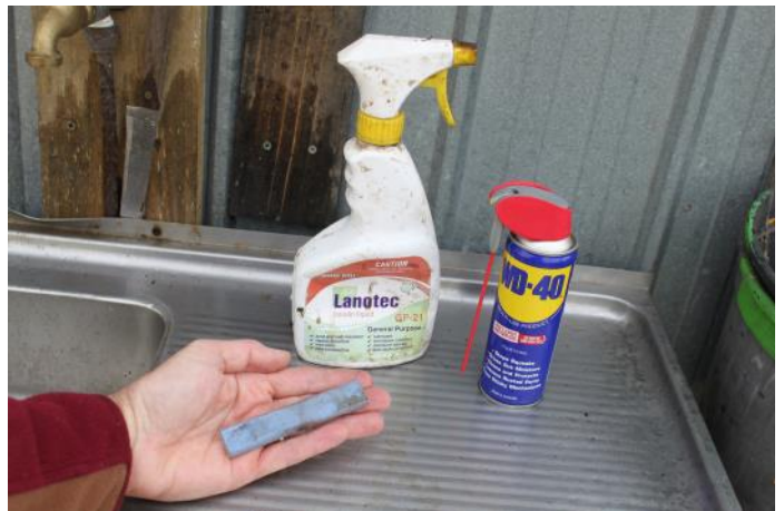
Felco grinding stone for sharpening knives and secateurs, Lanotec lanolin oil for oiling wooden handles and WD-40 for lubricating moving metal parts.
